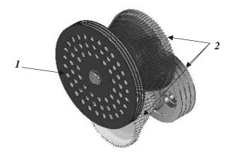
Fig. 9. Multi-disc corn grains new generation grinder construction unit -1, and gear systems -2 [1]
